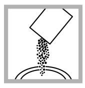
**5.** Add the contents of one Acid Reagent Powder Pillow for High Range Silica. A yellow color will show if silica or phosphorus is in the sample.
