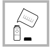
**10. Prepare the blank:** Fill a sample cell to the 10-mL mark with sample. Close the sample cell.
