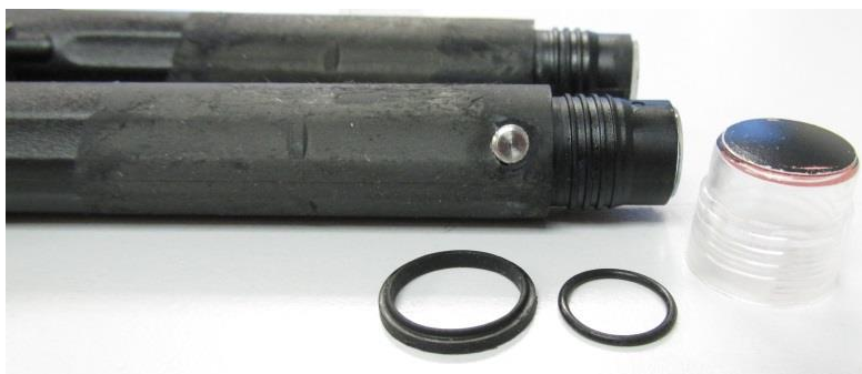
Figure 2: Damaged LDO probes in NaOH
