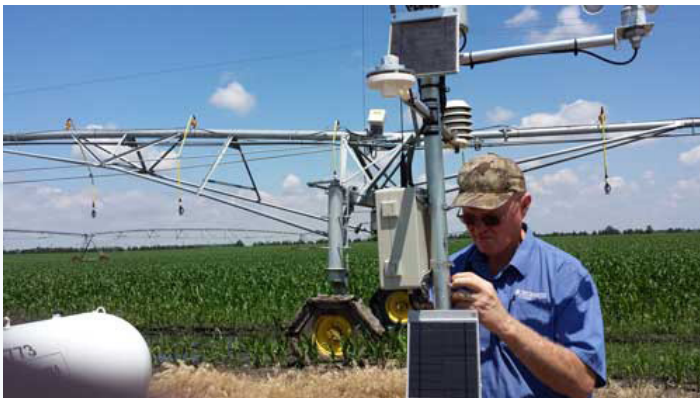
A McCrometer Regional Sales Manager installs a weather station for an agriculture customer in the Midwest. The weather station integrates various monitoring devices, including a propeller flow meter, to provide comprehensive farm data to the user.
