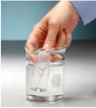
Fig. 7 Ampoule with dried reagent for quick check of \text{DO}_3 (Hach AccuVac)
