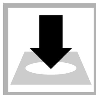
12. Insert the sample vial into the 16-mm cell holder. Make sure that the filter disc does not block the instrument light beam. Refer to [Before starting](#) on page 1.
