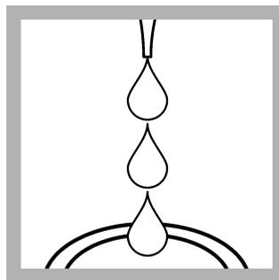
**3. Prepare the blank:** Use a pipet to add 9.0 mL of deionized water to a glass mixing cell.
