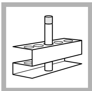
5. After an hour, remove the vials from the DRB200. Let the vials cool in a rack for two minutes. If the solution develops a colorless upper layer and a purple lower layer, invert the vials several times to mix.
