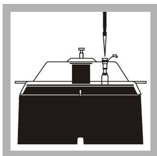
6. **Prepare the sample:** Use a pipet to add 0.60 mL of each acidified sample into the CRC.
