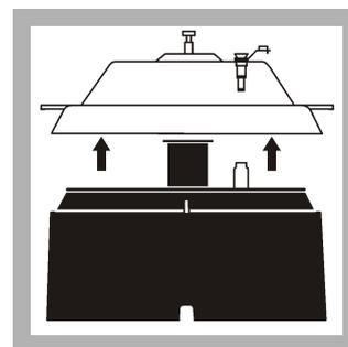
8. Open the VPD regulator to release the vacuum. Turn the pump off. Remove the VPD top and set it aside. Dispose of the used Chloride Removal Cartridges. Go to [Sample preparation and measurement](#) on page 5.
