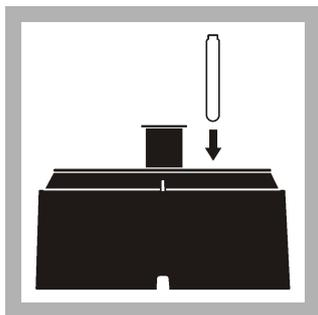
2. Write a sample identifier on each vial. Insert the Mn III COD vials in the numbered holes in the VPD base. Remove the caps from the vials.
