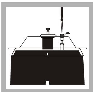
5. **Prepare the blank:** Use a pipet to add 0.60 mL of acidified blank into the CRC. It should take 30–45 seconds to pull the liquid through the CRC into the vial.
