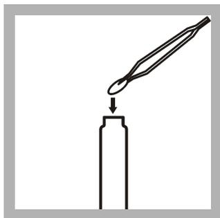
2. Insert each filter into the corresponding Mn III COD vial. Use the numbers on the VPD as a guide. Use a clean towel or deionized water to clean the forceps between samples.
