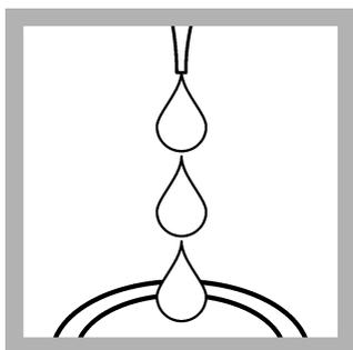
**5.** Use a pipet or dispenser to add 1.0 mL of concentrated Sulfuric Acid to both mixing cells.
