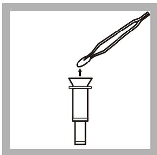
1. Use forceps to remove the filter from the top of the CRC. If the sample does not contain suspended solids, it is not necessary to transfer the filter to the digestion vial.
