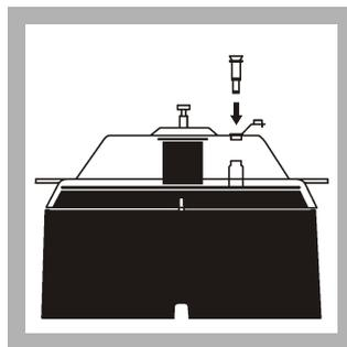
3. Put the VPD top on the base. Insert a fresh Chloride Removal Cartridge (CRC) directly above each Mn III COD Reagent Vial. Close any open holes in the VPD with the supplied stoppers.
