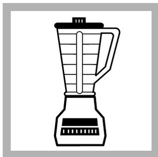
**2.** Put 100 mL of sample in a blender. Blend for 30 seconds or until homogenized.
