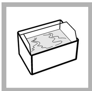
6. Let the vials cool to room temperature in a cool water bath, or hold under running tap water for several minutes.
