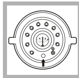
4. Start the vacuum pump. Adjust the vacuum regulator valve on top of the VPD until the internal gauge reads 20 inches of water.
