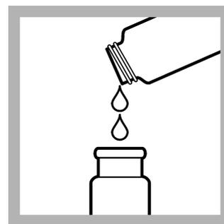
24. When the timer expires, pour the prepared sample and the prepared blank into two square sample cells. Let the sample cells stand undisturbed for 30 seconds to enable any turbidity to settle.
