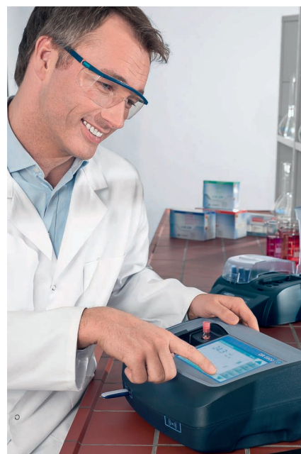
Measurement station for laboratory analysis, with DR 3900 photometer, LT 200 thermostat and LANGE cuvette tests
