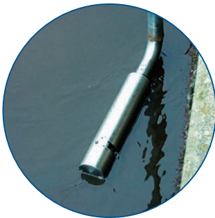
Partially immersed NITRATAX sc probe for online nitrate measurement
